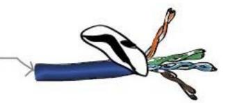
Untwist and flatten the individual wires.
